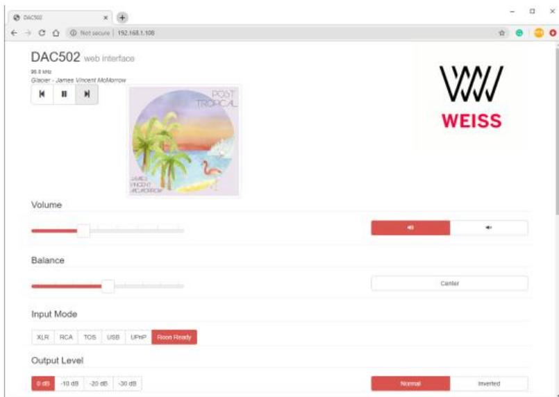
There are a total of five inputs: AES/EBU, Toslink, Coax, UPnP/DLNA, USB and Roon Ready. Accepted formats include PCM 44.1kHz up to 384 kHz and DSD 64x / 128x. The DAC has XLR and cinch outputs. The conversion is done via “two of the latest 32 bit D/A Converter chips”, interestingly, at a fixed 195kHz frequency which means that all the input signals are resampled to this frequency. According to Weiss, this helps significantly in reducing any jitter related effects. Included is an
